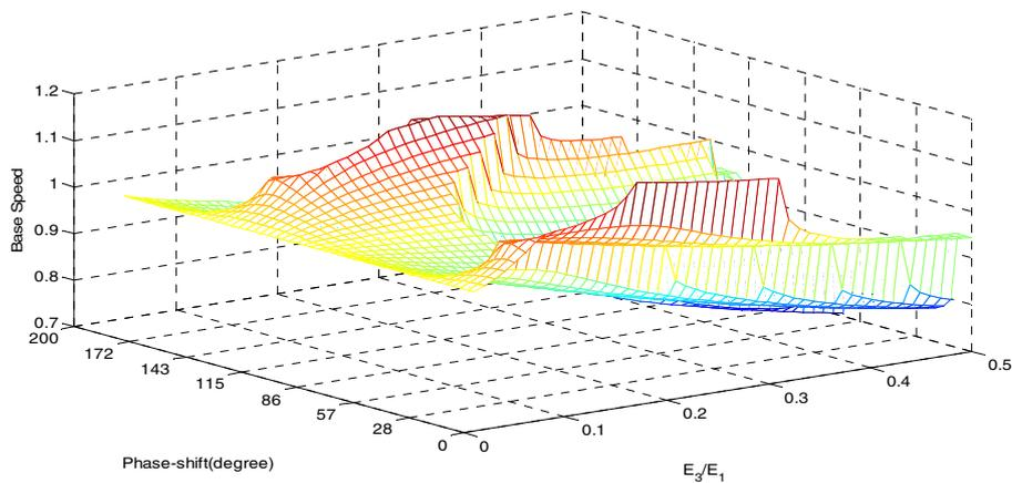
Figure 4 : Base speed according to  $E_3/E_1$  and phase-shift
