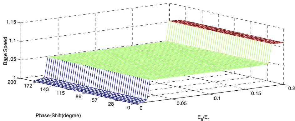
Figure 6 : Base speed according to  $E_3/E_1$  and phase-shift
