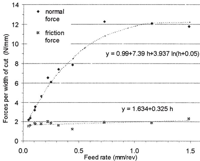
Figure 9. — Friction and normal forces  $F_m$  and  $F_{fr}$ .  $F_m$  and  $F_{fr}$  are resulting from the projection of the chip force along the rake face in parallel and orthogonal direction. Only values where the feed rate is equal to the tool-chip contact length have been considered.
