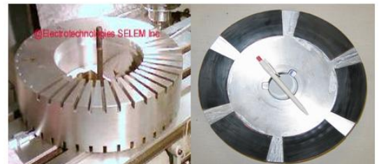
Fig. 2. Stator and rotor of the proposed machine.
