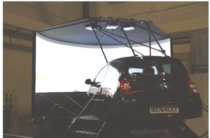
Figure 17. Operating of the dynamic driving simulator SAAM
