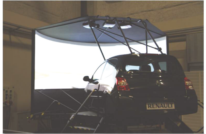
Figure 17. Operating of the dynamic driving simulator SAAM
