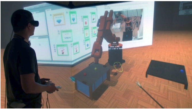
Fig. 8. Human controlled robot via high level speech commands
