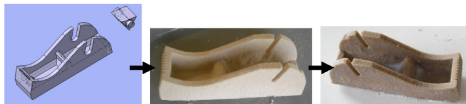
Figure 5 Scotch-tape support: computer-aided design model and manufacturing process (see online version for colours)
