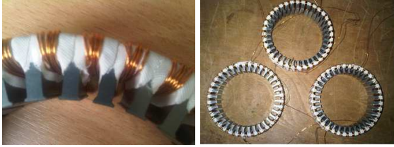
Figure 1: Samples of stators wound manually
