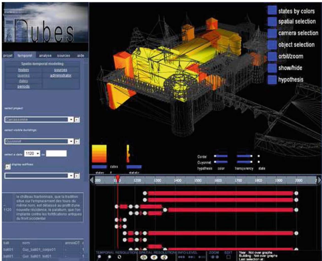
Fig. 17 NUBES web interface. The graphs on the bottom describe buildings lifespan and their “temporal position”
