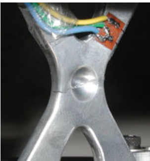
Figure 25: A biaxial fatigue specimen made from cast AlSi7-Cu0.5Mg0.3 showing that crack initiation did not occur in the biaxial zone in the centre of the specimen
