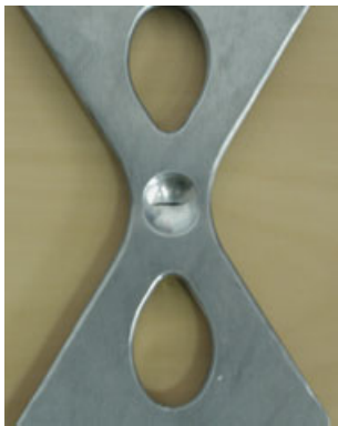
Figure 24: Typical fatigue failure of the biaxial specimen in Al 2024
