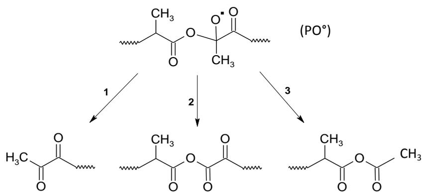
Figure 3: Possible  $\beta$ -scissions of the  $PO^\bullet$  radical according to [24].
