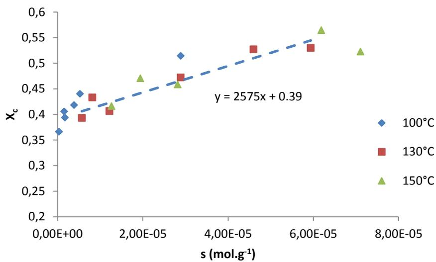
Figure 7: Degree of crystallinity as a function of the number of chain scission per mass unit.
