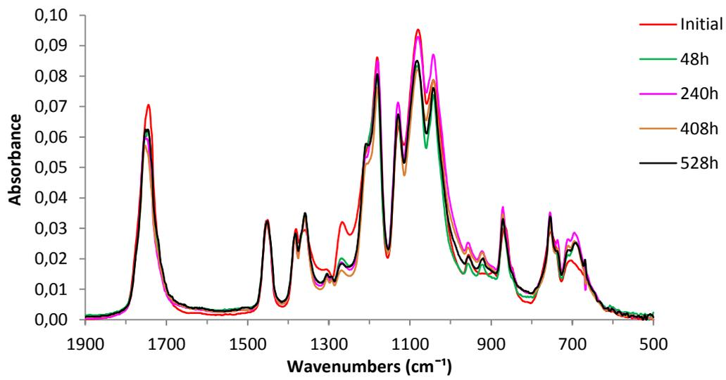
Figure 1: IR spectra of PLA films in ATR mode during thermal oxidation ageing at 150°C, (normalization at 1453 cm<sup>-1</sup> assigned to  $\delta_{as} CH_3$ ).
