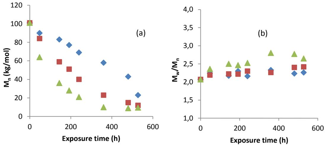
Figure 4: (a)  $M_n$  and (b) polydispersity index changes of PLA samples aged at 100 (◆), 130 (■) and 150°C (▲).
