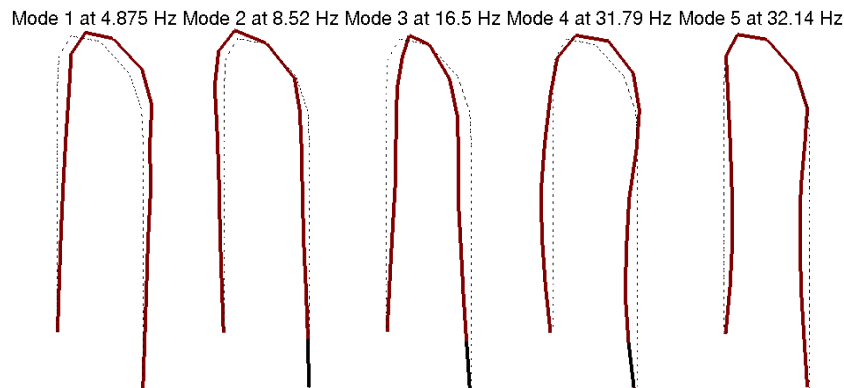
Figure 2: Experimental modeshapes of the free tube
