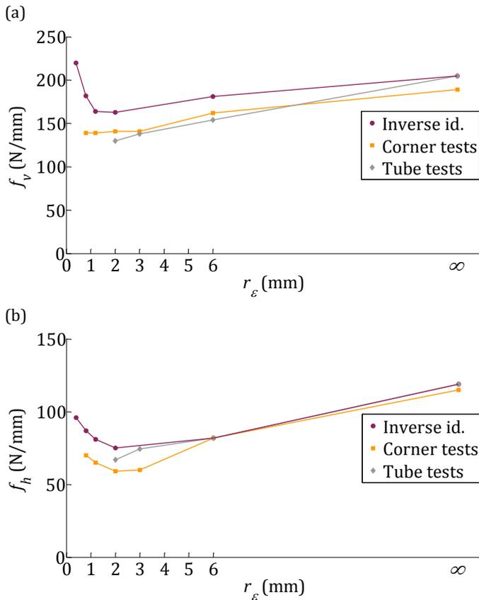
**Figure 4.** Comparison of the results of the three approaches, for the force components: (a)  $f_v$  (cutting force); (b)  $f_h$  (thrust force).
