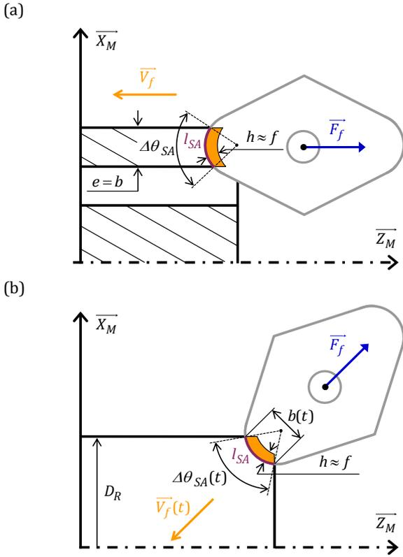
**Figure 3.** Configurations of the elementary cutting tests in the nose: (a) Tube; (b) Corner.
