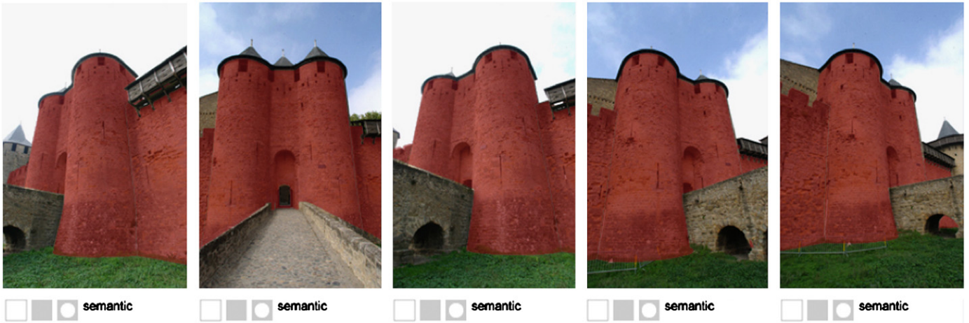
Fig. 12. Entity-based images searching in the 3D scene. When one or more 3D entities are selected in the 3D scene, all photographs in which these elements are present are listed. The semantic layer related to the selected elements (mapped on photos as a SVG mask) is highlighted.
