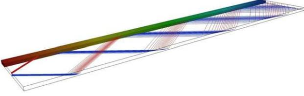
**Fig. 9.** Computed pressure field and flow pathlines for a two-ply rectangular laminate  $1 \text{ m} \times 0.2 \text{ m} \times 0.01 \text{ m}$ ,  $\Delta P = 0.05 \text{ bar}$  with  $45^\circ / -45^\circ$  orientation.
