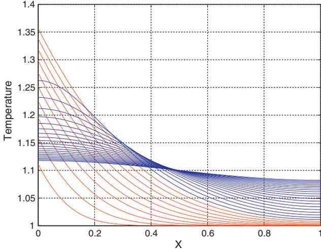
**Fig. 1.** Temperature profiles corresponding to the source term (13) at discrete times  $t_m = m$ , for  $m = 1, 2, \dots, 30$ . The red curves correspond to the heating stage up to  $t = 10$ , while the blue curves for  $t > 10$  illustrate the heat transfer by conduction from the warmest zones towards the coldest ones. (For interpretation of the references to color in this figure legend, the reader is referred to the web version of the article.)
