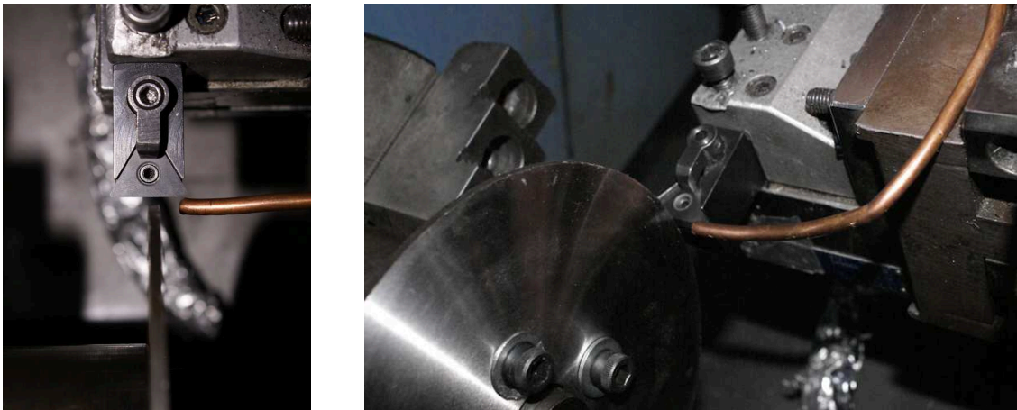
Figure 1. Experimental set-up: orthogonal cutting with cryogenic delivery nozzle position [12].
