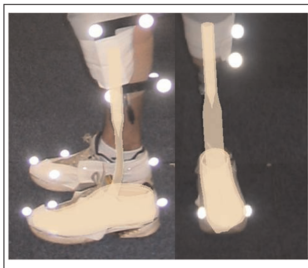
Figure 2. Registration of the digital model of the prosthetic foot on the calibrated photographs.
