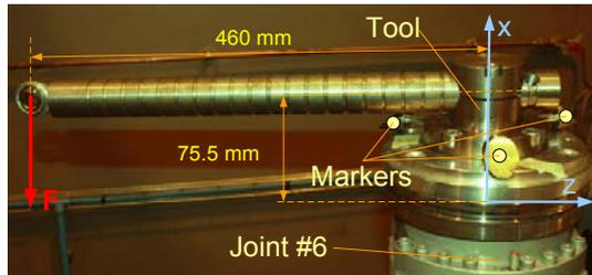
Fig. 2. End-effector used for elastostatic calibration experiments
