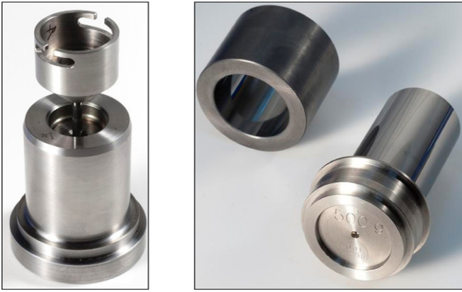
Figure 1. Piston and cylinder of a pressure standard piston–cylinder assembly.
