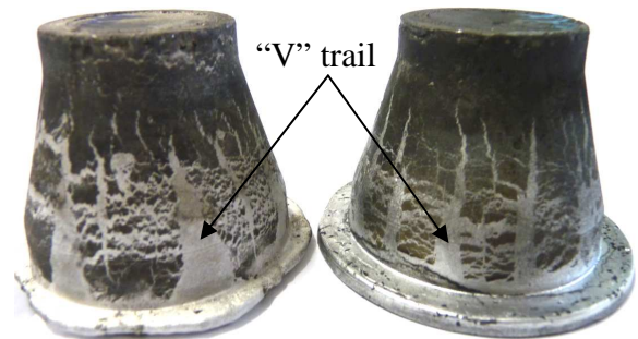
Fig.7 Parts thixoextruded at 615°C: working ram speed a) v=235 mm/s; b) 416 mm/s.
