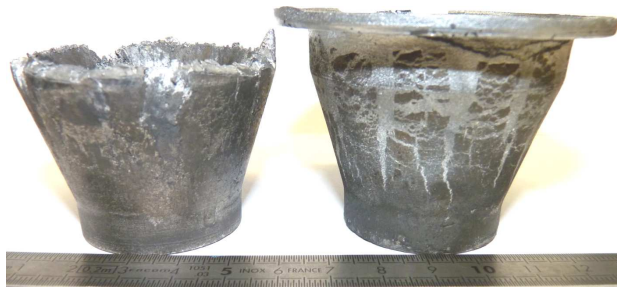
Fig.9 Parts thixoextruded at 590 °C and 620 °C
