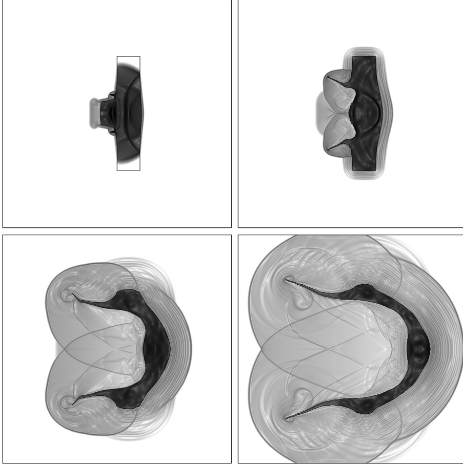
Fig. 24. Impact of a projectile on a plate for \chi = 0 (TC11). Numerical Schlieren pictures at t = 38 \mu\text{s} , 140 \mu\text{s} , 420 \mu\text{s} , 710 \mu\text{s} .
