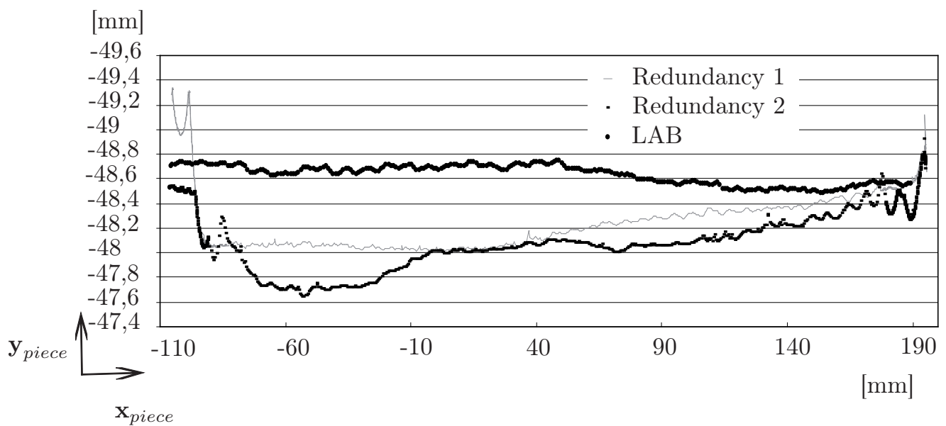
Figure 4.7 – Quality of the test workpiece milled in a given placement, but with two different redundancy planning schemes
