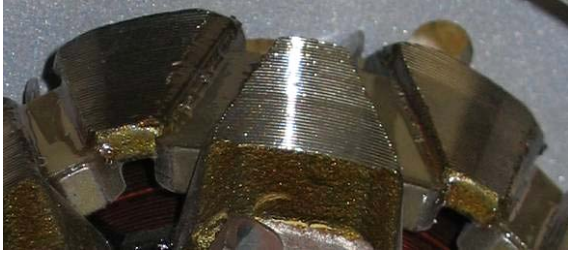
Figure 1. Picture of a claw-pole rotor with permanent magnets inserted between the claws
