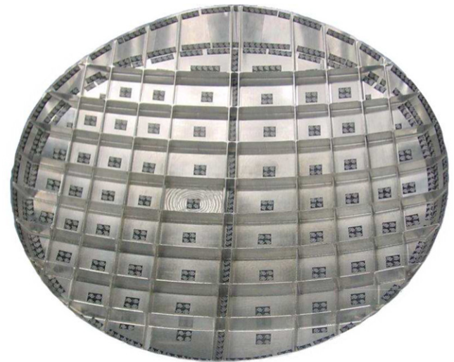
Fig. 7. Prototype of a forward pressure bulkhead.
