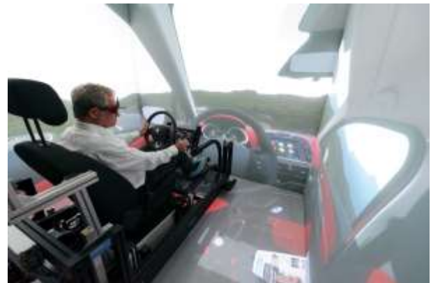
Figure 5. Renault's high performance CAVE™ with driver station
