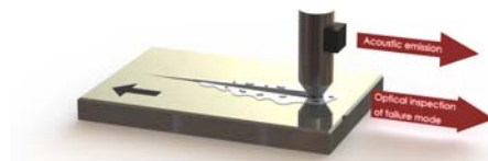
Figure 1. Scratch test device
