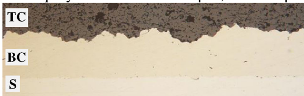
Cold spray BC: thickness 220μm, Ra=12.2μm
