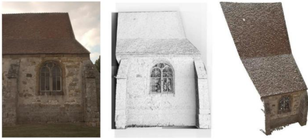
Figure 2: The multi-stereo image matching method: the master image (left), the matching result in the last pyramidal step (center) and the generated colorized point cloud (right)
