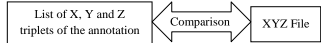
Figure 10: A comparison between the list of X, Y and Z triplets of the annotation and the XYZ files helps to project the annotation on the other images
