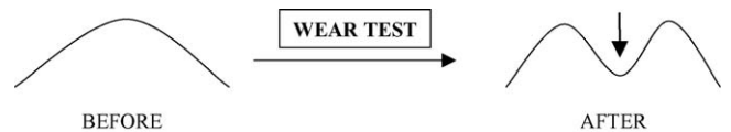
Fig. 6. Schematic representation of the effect of hard abrasive particles acting at the top of a soft asperity during a wear test. A black arrow highlights the location where an abrasive particle penetrated at the top of the asperity. At a microscopic scale, this ploughing effect results in an increase of the number of inflexion points of the profile and therefore of the chaotic aspect of the profiles.
