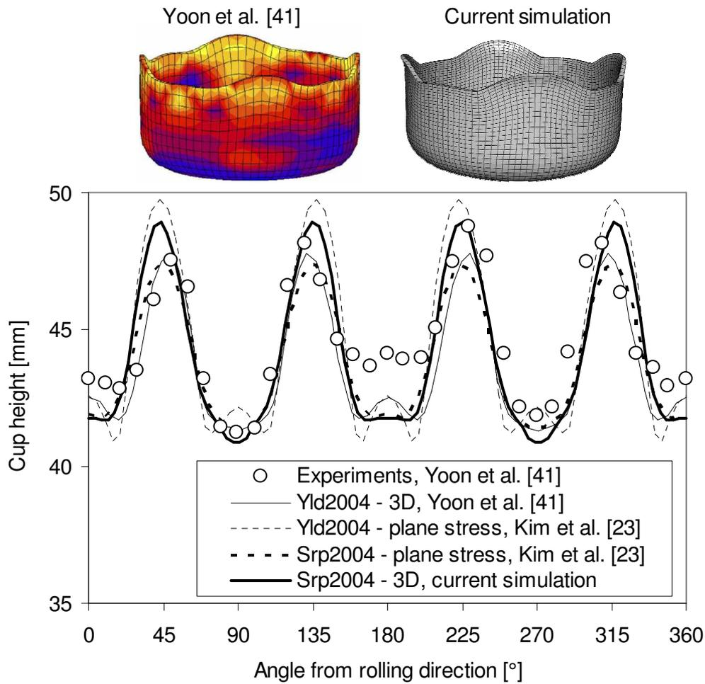
Figure 5. Results of the numerical simulation of cup drawing with Srp2004-18p; cup height profiles for the current simulation and the reference simulations in [41] and [23], compared to experiments.
