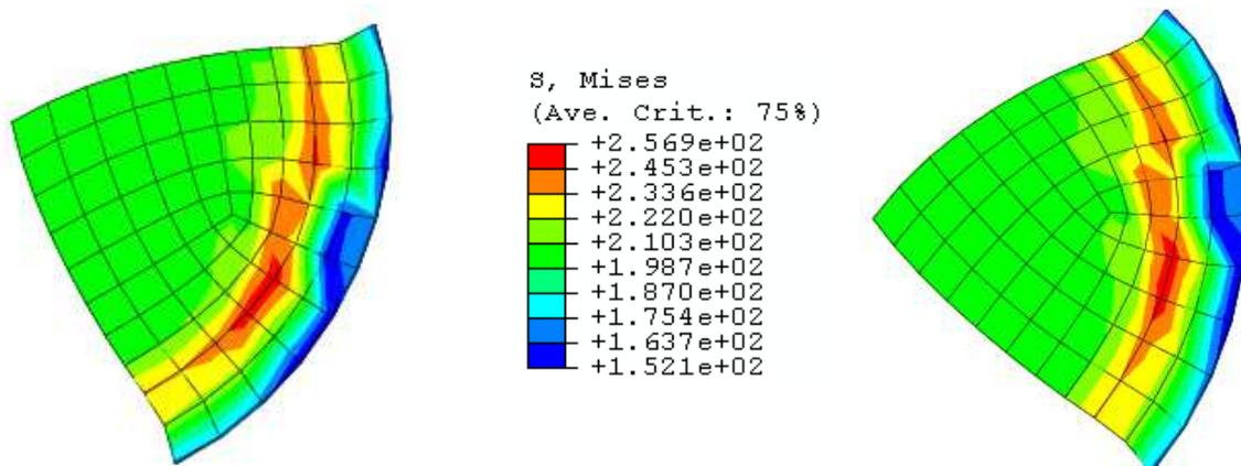
Figure 2. Finite element simulation results for the bulge test. Left: using the Abaqus/Standard built-in model and algorithm; Right: using the current model and algorithm implemented in Abaqus/Standard via UMAT. Isovalues of equivalent stress.
