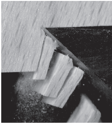
Figure 6: Results of high speed milling experiment on green beech ( V_c = 420 m/min, h = 10 mm).
