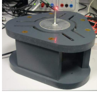
Fig. 16. Speed measurement by a laser vibrometer
