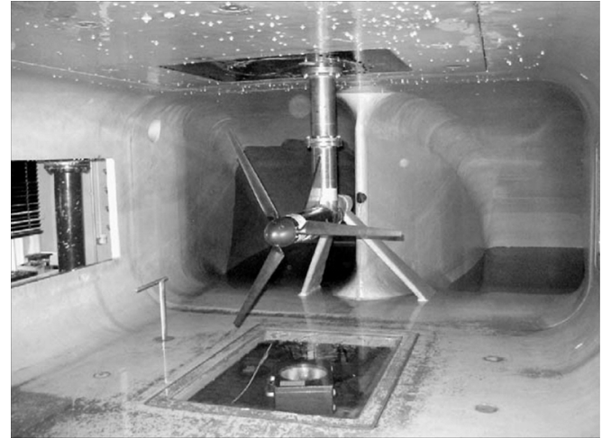
Fig. 13. Marine turbine tested in [39]. (Illustration reproduced with the kind permission of the authors.)
