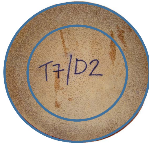
Figure 1: Coconut disc showing that the most valuable area for high density veneer production lies between the blue circles
