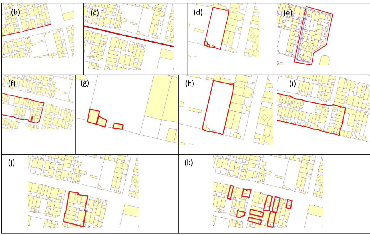
Fig. 3. (a) The ontology of the urban environment layouts describing the components of a city and an illustration of (b) edge, (c) path, (d) parcel, (e) urban area, (f) block (isolated parcels), (g) building lot, (h) parcel boundary, (i) district (parcel set), (j) parcel set (parcels with connections to others) and (k) parcel set (separated parcels).
