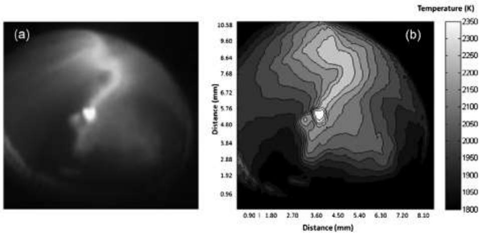
Figure 6. (a) Convex weld pool, and (b) calculated thermal field at the surface.
