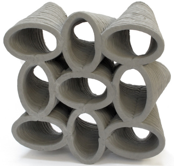
Fig. 8. Concrete 3D printed acoustic damping wall element.
