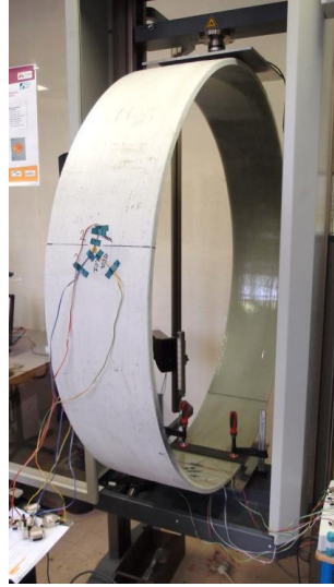
Figure 2. Radial compression set-up.
