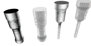
Fig. 2. Meshed models of the tools and their voxelized counterparts at a resolution of 0.5 voxel per micron.
