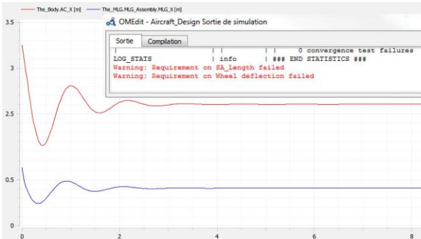
Figure 17 The monitoring performed by a specification model signals the violation of two PBRs
