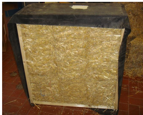
Figure 11. Full size test sample prepared for thermal conductivity measurement.
