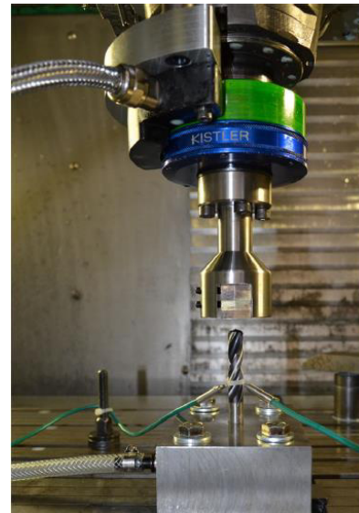
Fig. 3. Drill instrumentation with thermocouples type K for temperature measurements. T1 and T2 show the location of the thermocouples [8].
