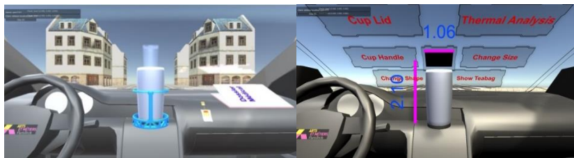
Figure 5: An example of using multi-view system in the product (mug) design. Left picture: the scenario of utilization in a car. Right picture: the panel of tools available for the designer.
