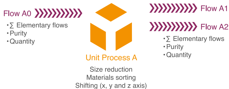
Figure 3 Modelling of a recycling pathway step with a separation unit process
