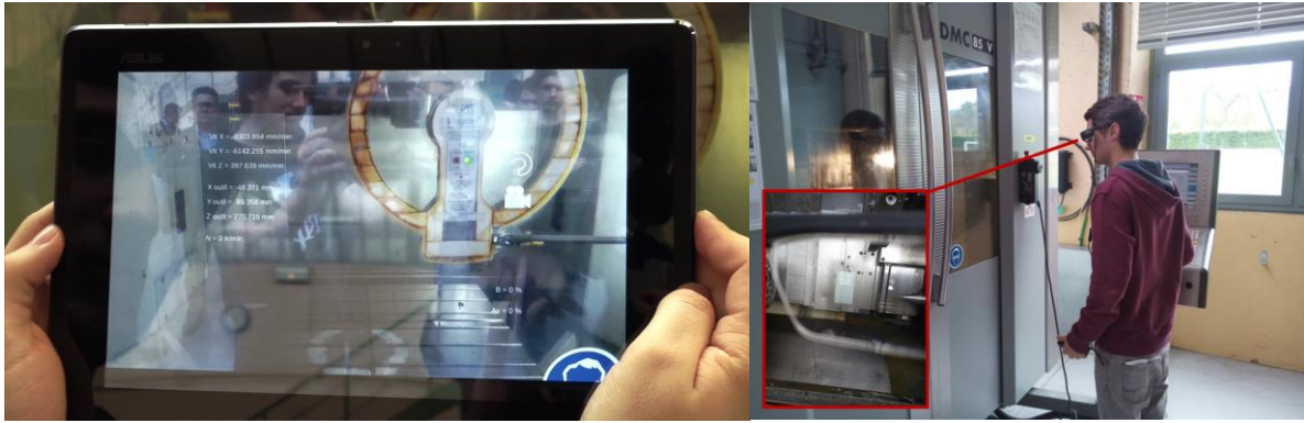
Fig. 4. AR system in operation (on the left: using a tablet PC; on the right: using AR glasses with a zoom on displayed information)
