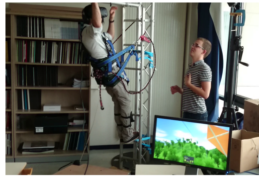
Figure 2: The work-at-height simulator in operation.
