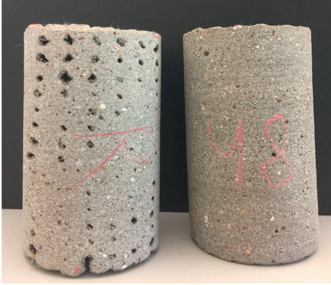
Fig. 7. Two samples that represent good quality printing on the right and poor quality on the left. On the left, the outline of each filament can be identified, interspersed with inter-filament voids of various sizes, whereas the filaments are indiscernible in the right hand sample.
