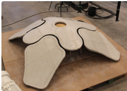
a) a panel, horizontally printed, shell and fill application. Image: 4TU project 3D printing on flexible mould TU Delft and TU Eindhoven, Netherlands.
