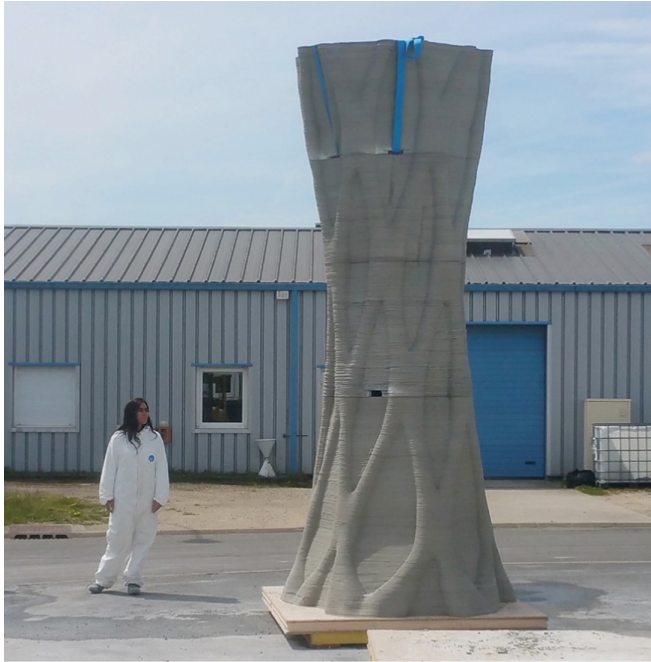
Fig. 8. Assembly trial after printing of the four parts.
