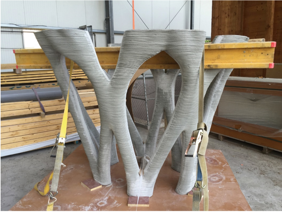
Fig. 10. Cast and lost formwork assembly from which the printing supports were cut.
